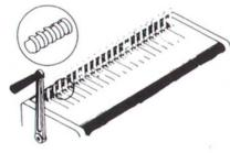
Turn clockwise to open, pull handle to desired opening, then turn knob counter-clockwise to lock.
